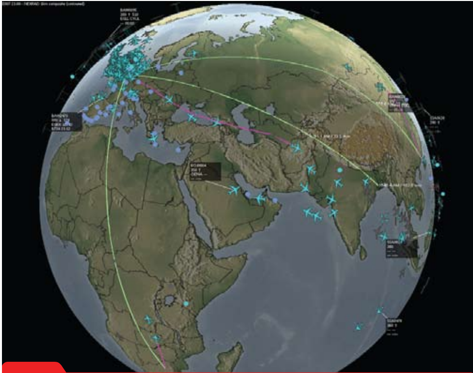
Flight Explorer enables airlines to track aircraft anywhere in the world. Both ATC radar data and ACARS information is used to graphically display aircraft in real time so an airline always knows the locations of its aircraft.
