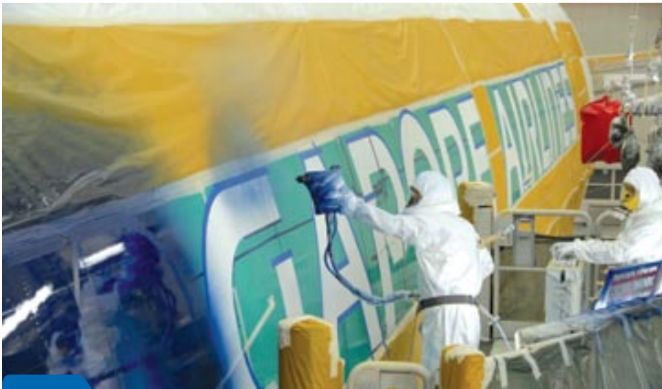
The painting of Singapore Airlines' first A380 took 21 days and used more than 2,200 liters of chromate-free paint.
