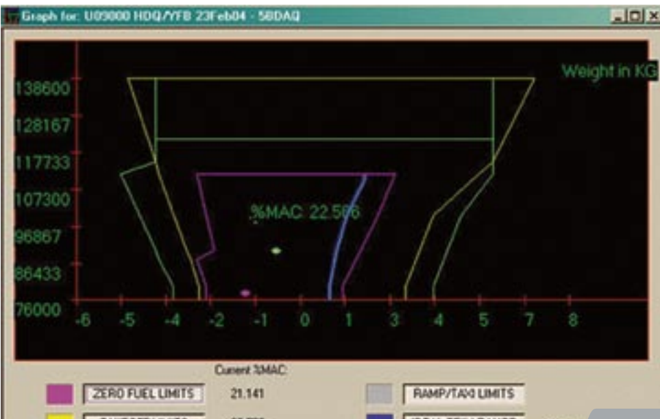
The load planner can easily choose one or all limits to display by clicking the desired limit button. The chart is a powerful tool in which the load planner can view the weight and balance envelope at any time of the load planning process.
