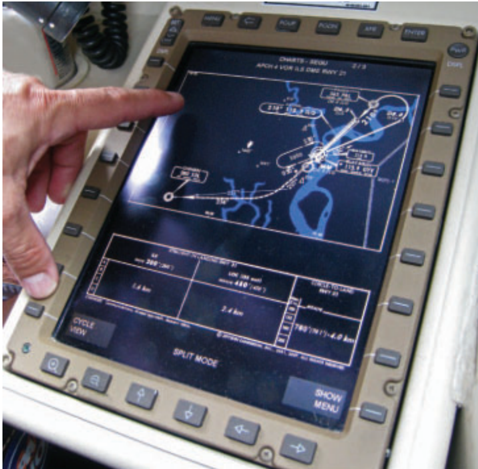
An Electronic Flight Bag includes all documentation and forms carried by pilots, such as aeronautical charts, manuals for fault reporting and operations, minimum equipment lists, and logbooks. Its weight-and-balance calculator enables pilots to instantly determine the ideal speeds and engine setting for an aircraft, in any weather, on any runway, with any payload.
