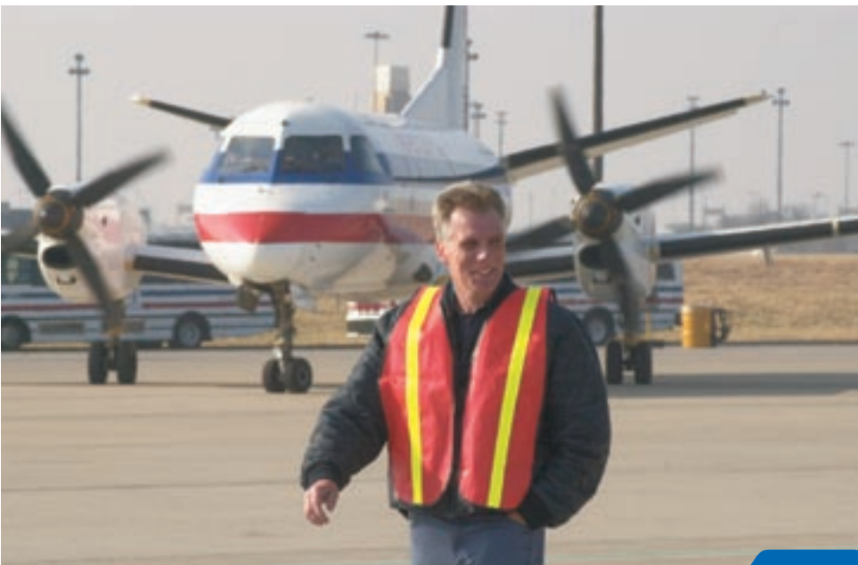
To decrease fuel consumption, ramp employees avoid making planes wait to be wanded in as well as promptly hook up electrical and ground air upon arrival. They also shut down any ground equipment while not in use.
