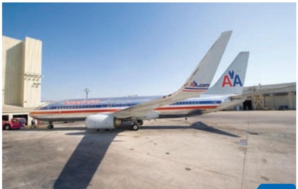
By adding winglets to certain aircraft, such as the Boeing 737 and Boeing 757, as part of its Fuel Smart program, American Airlines stands to save 25 million gallons of fuel annually.
