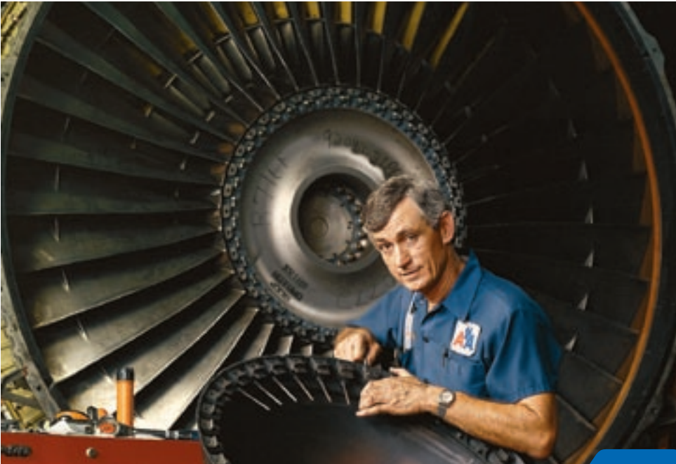
American Airlines' mechanics take every cost-saving measure to ensure aircraft are flown with utmost efficiency. Regularly cleaning aircraft engines, which improves fuel burn, saves the carrier 3.9 million gallons of fuel a year.
